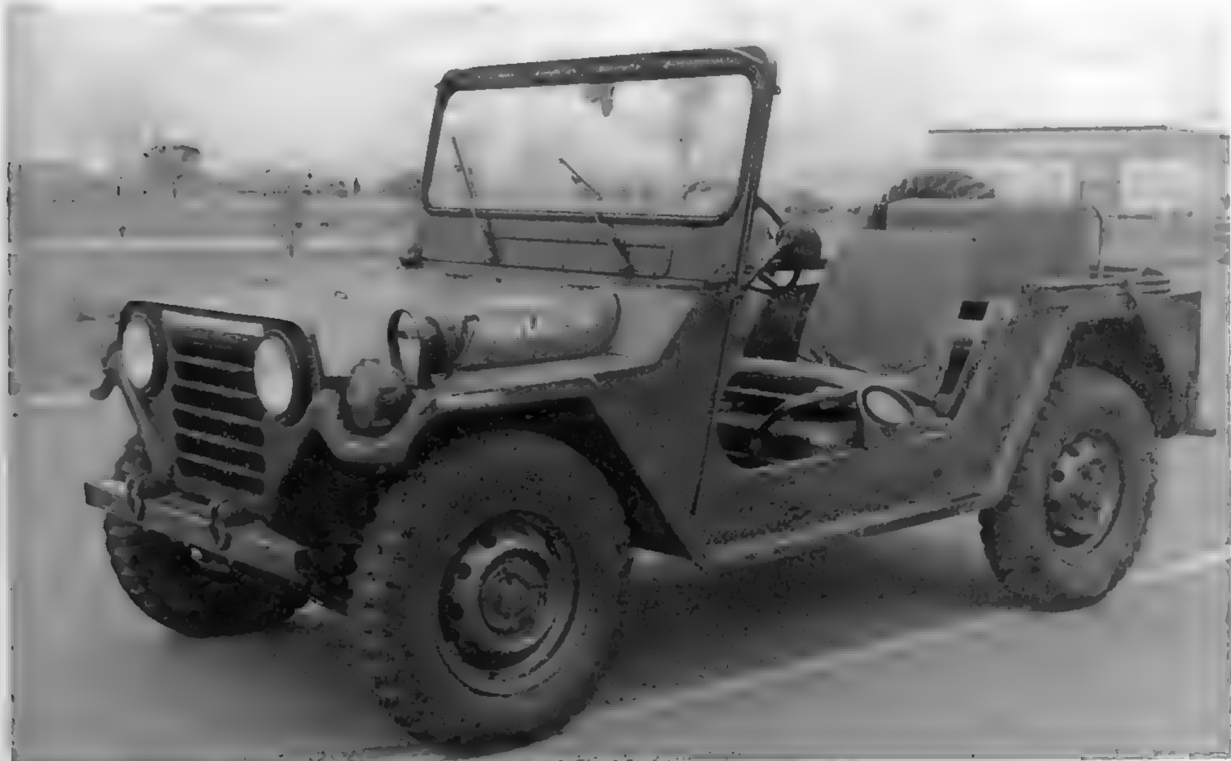
The M151A2 has scooped front fenders and a single-piece windshield. Underneath, there was a much-improved and safer suspension system. (U.S. Army photo)
